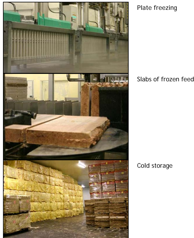
Figure 5 Feed production: plate freezing and storage
